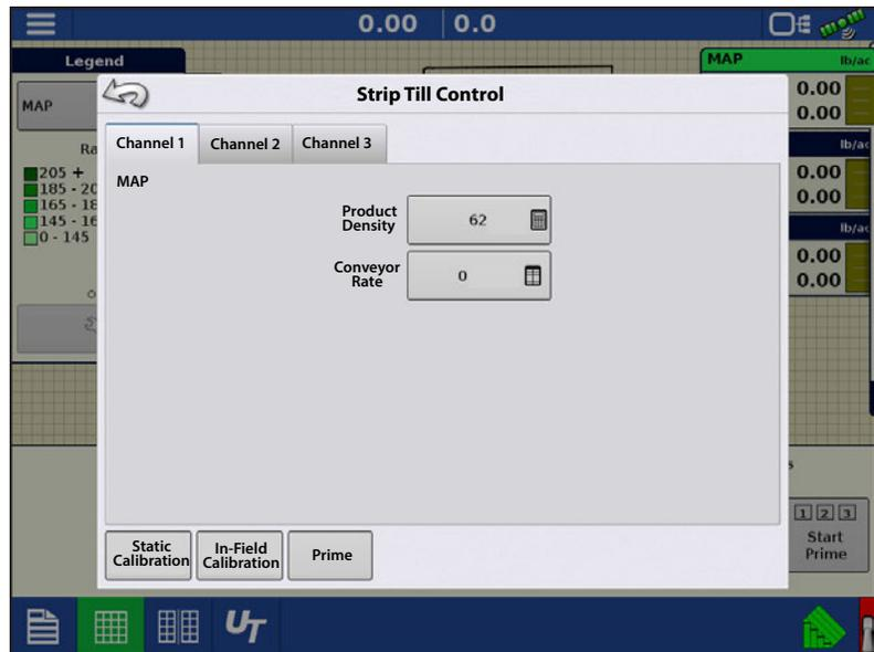
**Static Calibration**—Press the Static Calibration button to perform an automated routine to calibrate each metering circuit. This calibration is performed before applying in field conditions.
