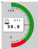
• When an Anhydrous Ammonia system is setup, NH<sub>3</sub> state monitoring is capable. In order to use the on screen gauge for NH<sub>3</sub> state monitoring, a temperature sensor and main line pressure sensor must both be installed and calibrated. Once both sensors are installed and calibrated, the UT pressure gauge will now display only RED and GREEN portions.
