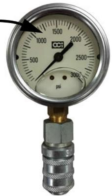
5. Screw the allen head adjustment IN to increase pressure sent to actuators; screw OUT to decrease pressure. Pressure (PSI) sent to actuators is shown on the pressure gauge.
