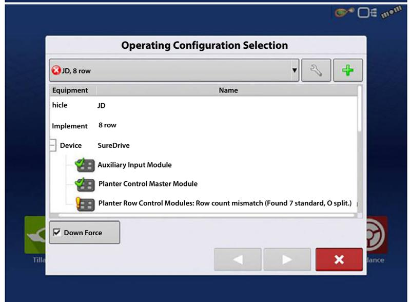
Image 3 - The message that will appear when there is an actual Split Row Mismatch due to a bad jumper in one of the interplant row modules.
