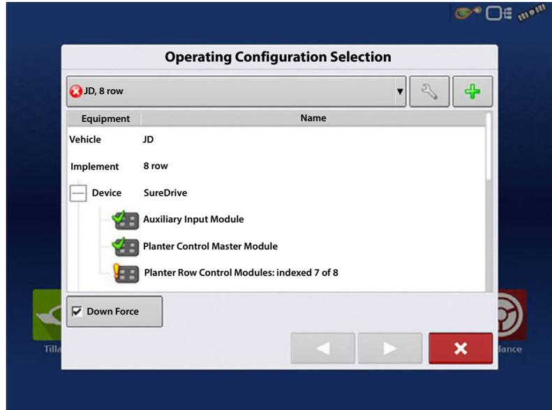
Image 2 - The message that will appear when there are more modules on the CAN bus than what the config requires.
