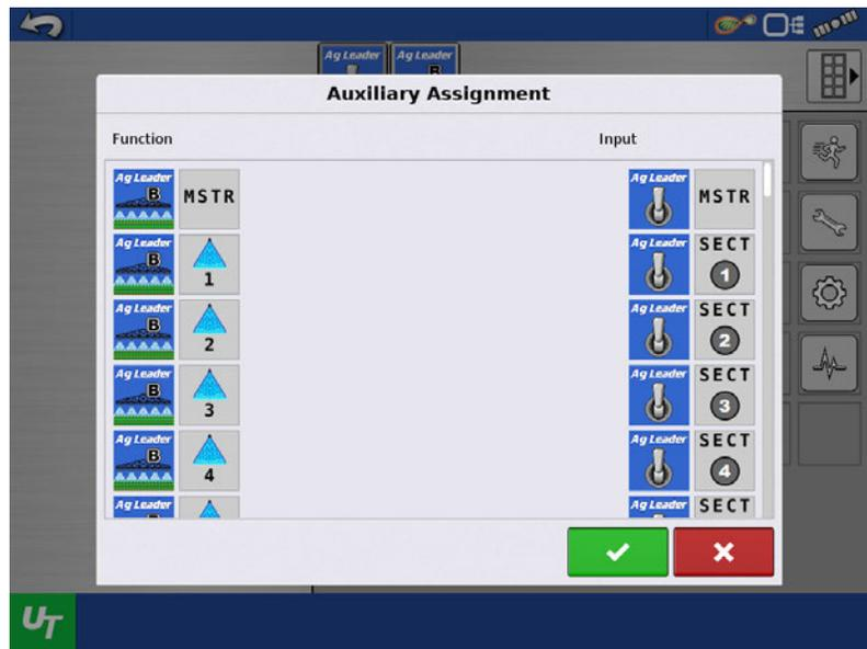
When using the SC7 Switch Console, the Rate Change and Increase/Decrease toggle switches can be assigned to a function. To assign these toggle switches, scroll down the Auxiliary Assignment page to locate the corresponding icons. Press the disconnected chain icons to assign the appropriate input. (See images on the right)
