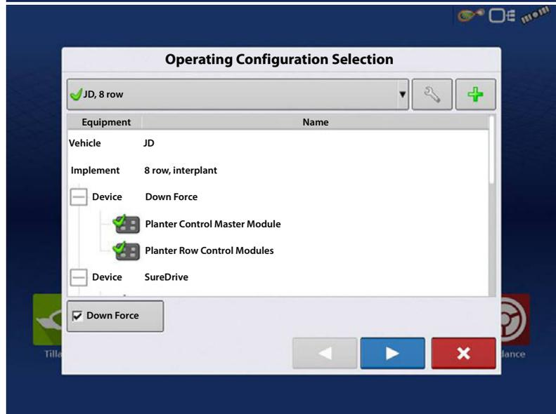
SureForce™ uses sensors to measure the weight carried by the gauge wheels. This information is used to adjust the down force so the planter is firmly on the ground, ensuring correct planting depth and reducing the risk of compaction. Individual Row Hydraulic Down Force control is only available with the InCommand™ 1200 display.
