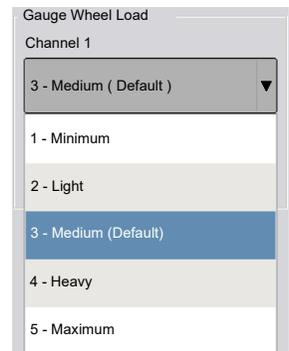
Target gauge wheel load will be overridden by SureForce when ground contact measurements are less than target. Ground contact is determined by monitoring gauge wheel load over time as the planter travels through the field.
