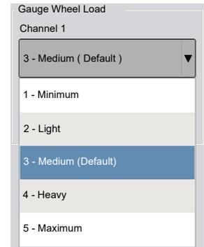
Example: Based on the ground conditions in a specific area of a field, the down force system applies 150 lbs of supplemental force in order to achieve a target gauge wheel load of 100 lbs. However, if the Gauge Wheel Load setting is set to **Heavy**, the target gauge wheel load is now 150 lbs. The supplemental force will adjust accordingly in order to achieve the new target gauge wheel load. (Keep in mind, the target gauge wheel load is a continuously calculated value.)
