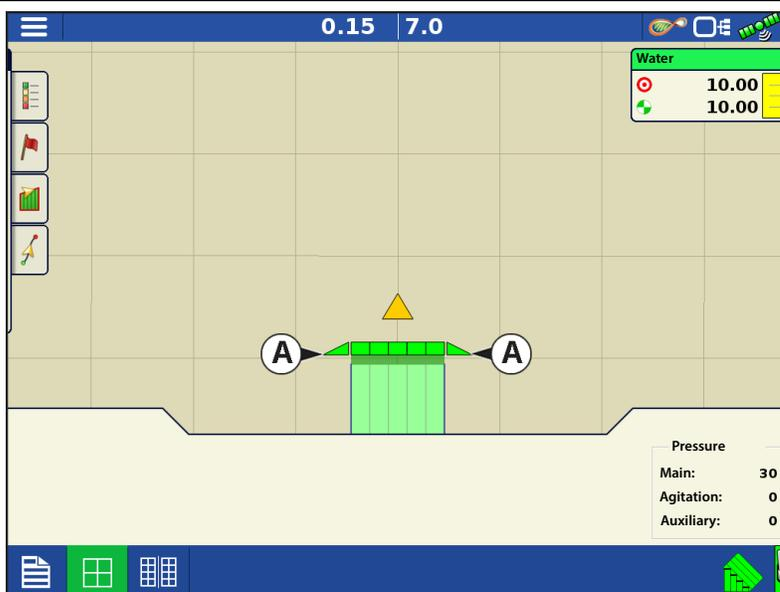
**i** NOTE! If a switch is selected as a Left or Right Fence Row Nozzle, the system sends power out of Boom Pin 11 for the left fence row, and Boom Pin 12 for the right fence row.
