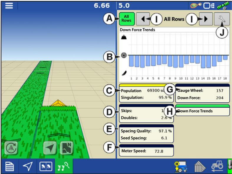
Advanced Seed Monitoring provides planter performance monitoring of seed meter singulation, skips/doubles and spacing quality, along with population and spacing information for all rows when planting compatible crops.
